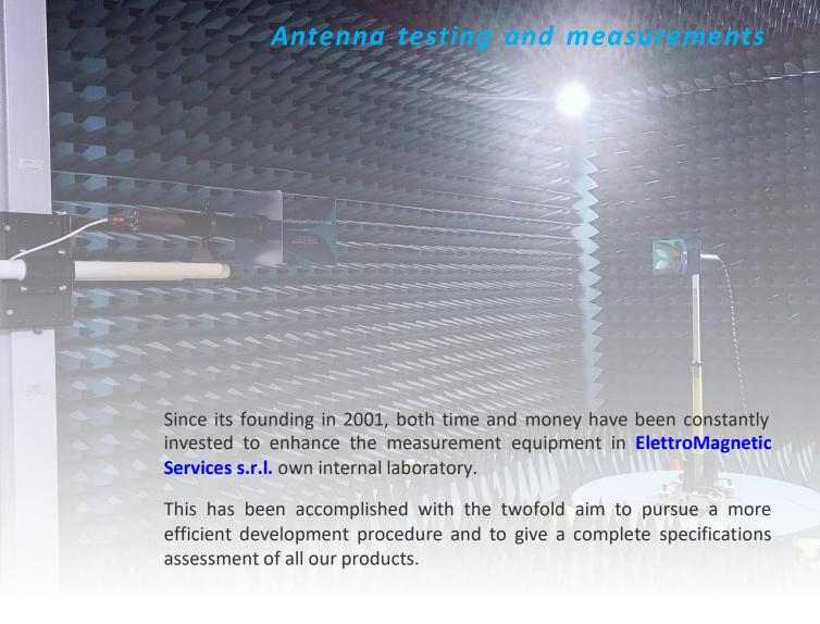
Now the company's laboratory includes an anechoic chamber with a fully automatic acquisition system that drives a rotary platform capable of a position accuracy down to 0.1 degrees. In this way it is easy to carry out precise radiation measurements also on antennas that are integrated into large housings or subsystems.
