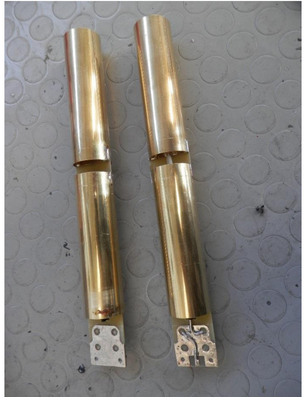
Figure 1 Constructive example of UHF radiating elements
