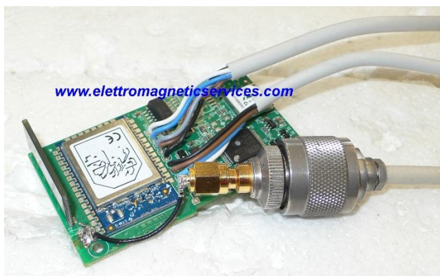
Preliminary measurements on a pre-existing integrated antenna, in order to determine reference specifications against which improvements can be made.
