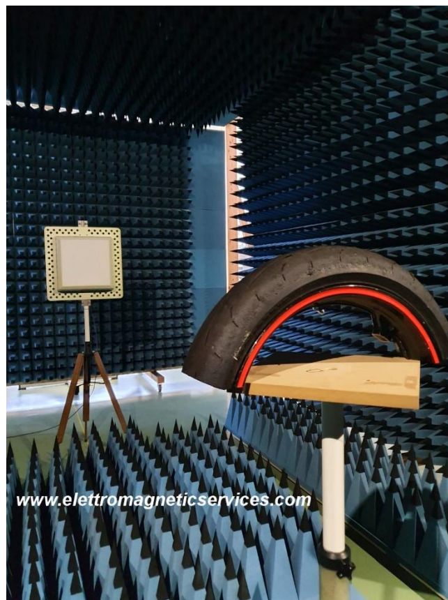
Measurements on an integrated antenna in a TPMS (Tyre Pressure Monitoring System) device for sports motorcycle tyres.
